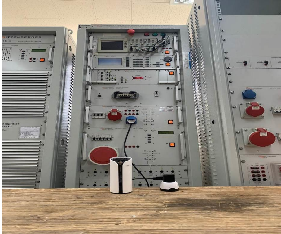
Photo of test setup for Voltage Fluctuations And Flicker
