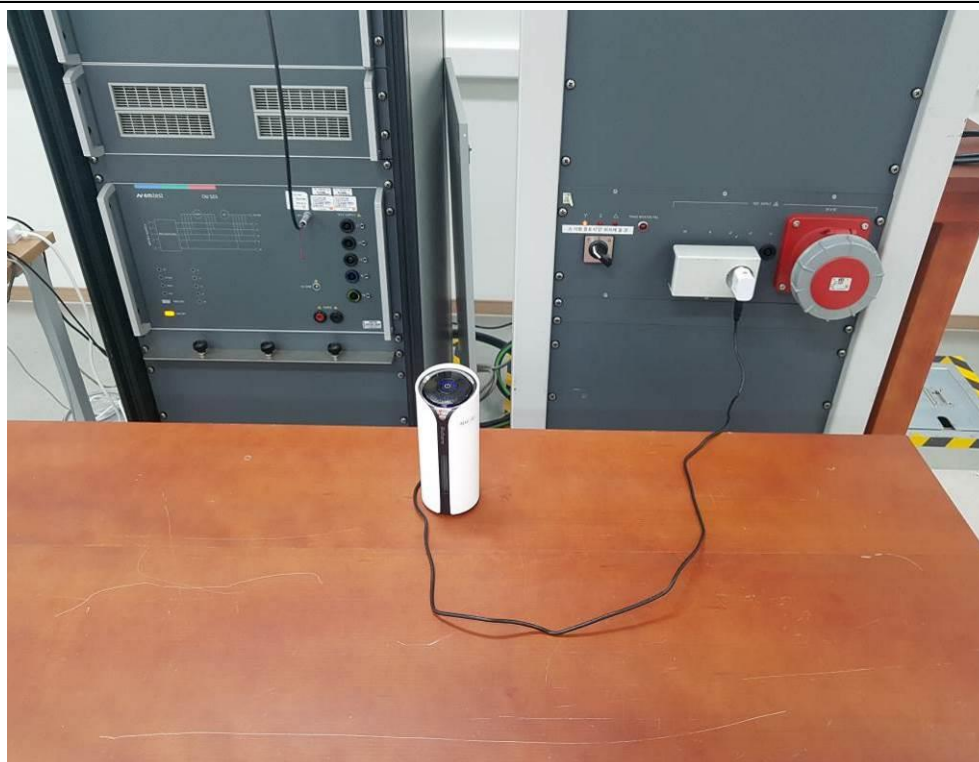
Photo of test setup for Voltage Dips, Interruptions, and Variations
